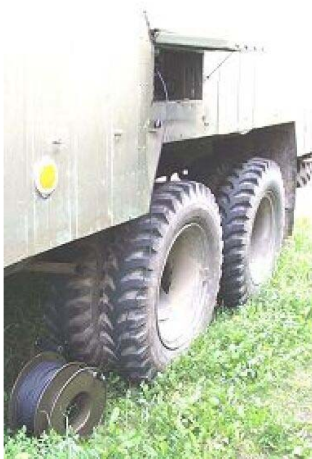
Figure 3-5: External Cable Panel with Connected FO Cable (on the reel).
