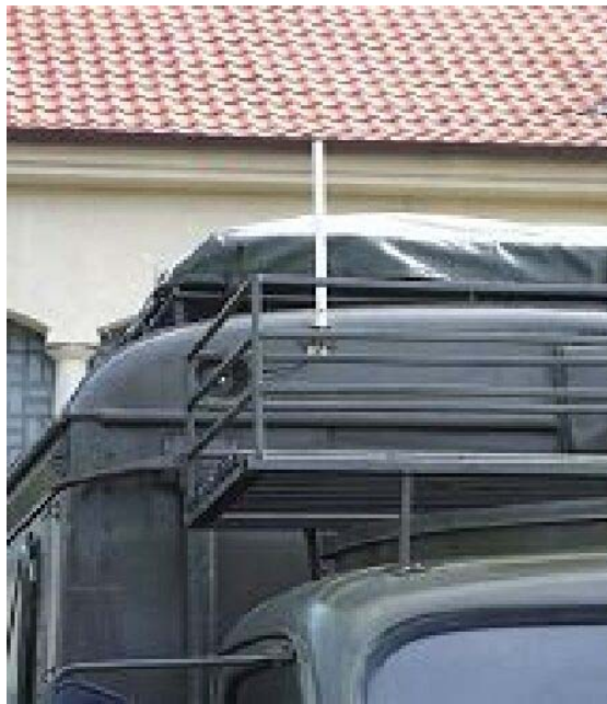
Figure 3-4: Detail View of Omni-Directional Antenna for WLAN on the Roof of Staff Shelters.
