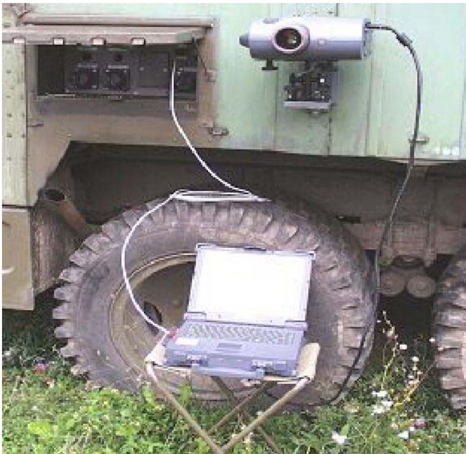
Figure 3-7: Connection of External Notebook GETAC with Data Projector to Shelter Cable Panel.
